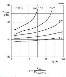
Fig 9. Drain-source on-state resistance as a function of drain current; typical value
